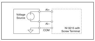
Figure 4. Connecting a Grounded Differential Voltage Signal to the NI 9215 with Screw Terminal
